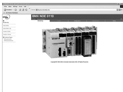
Modicon M340 hardware configuration
